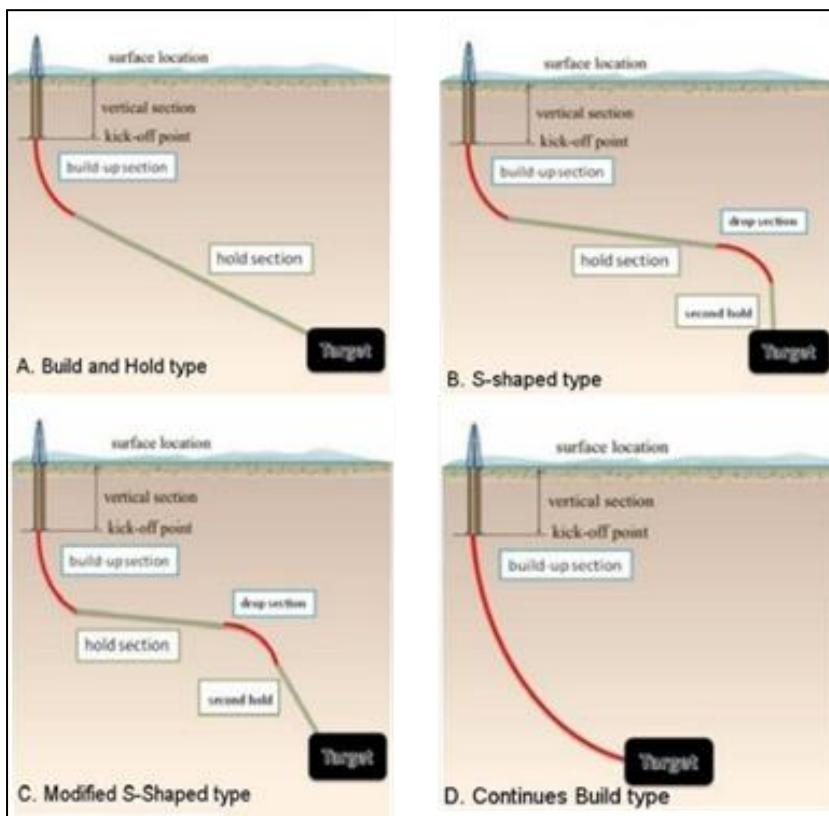
Gambar 1. Tipe Sumur Directional Drilling (Musa et al, 2017)
