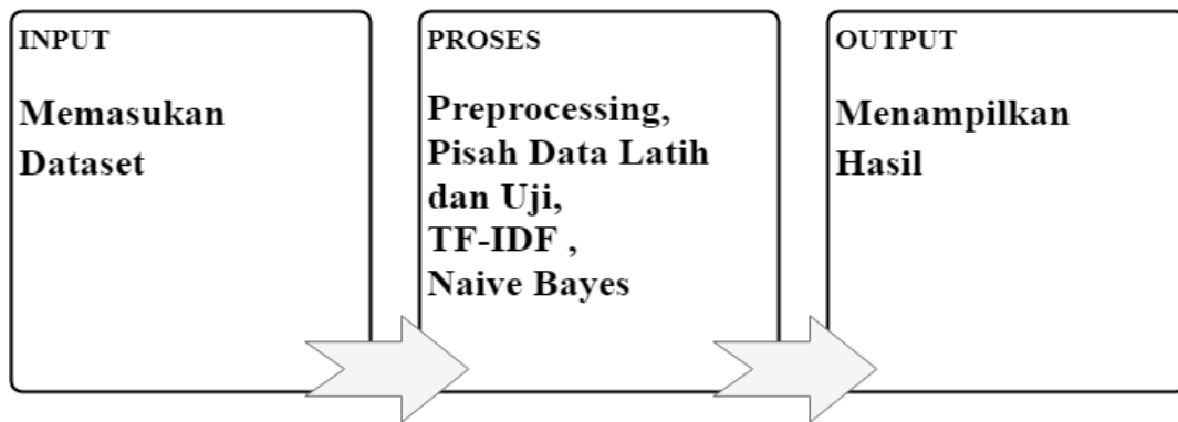
Gambar 3. Blok Diagram Program
