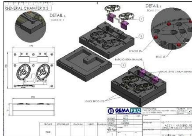
Gambar 6. Desain Prototype Jig Masking Mark Steering T
