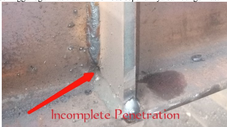
Gambar 2. Cacat Las Incomplete Penetration
